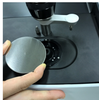
Fig. 3 Removal of ATR Crystal
