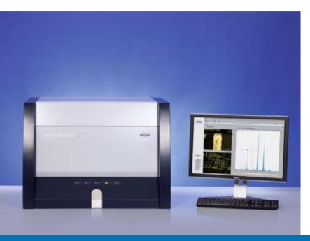
μ-XRF is the method of choice for highly sensitive and non-destructive elemental analysis of diverse samples, including inhomogeneous and irregular shaped specimens.
