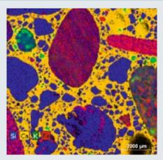
Fast mapping of a concrete sample (1 cm<sup>2</sup>) with 1 ms dwell time per pixel. Total measurement time: 3 min.
