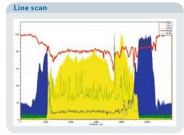
The Line scan shows the relative intensity distribution of selected elements on the inclusion of an iron meteorite.
