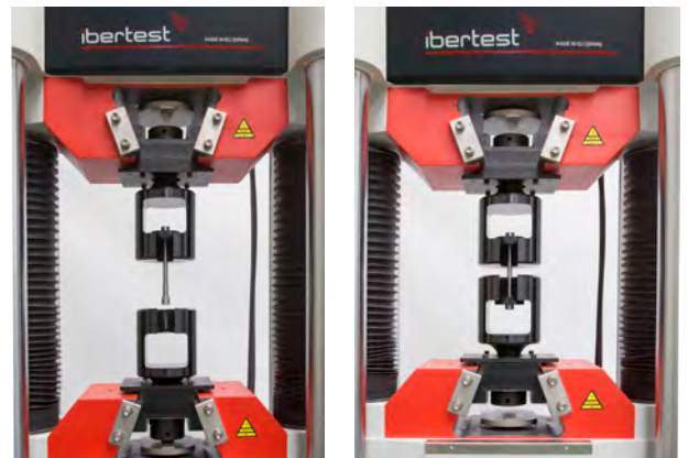
Accessory: tensile device for cabezales for button or/and threaded shouldered metallic specimens
